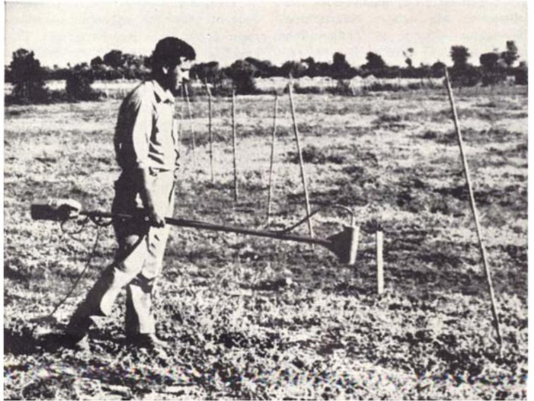
Fig. 6. Beginning a rubidium magnetometer traverse over grid 16 of the exploration site. The area is underlain by a complex of structures at a depth of 3 to 6 meters
