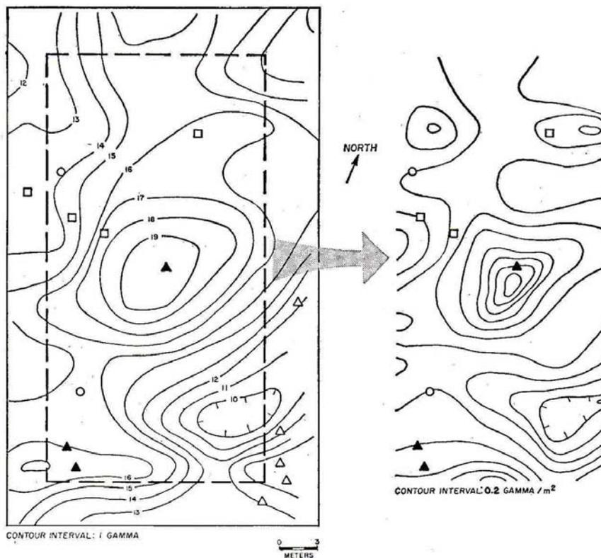
Fig. 9. (Left) Plot (grid 15: Zona Casa Bianca, plain of Sybaris, October 1964) of total magnetic intensity over ruins buried at depths of 3.5 to 6 meters, and results of drilling. (Right) Plot of computed second vertical derivative for the area outlined by dashed lines in the plot at left. (Circles) No results; (squares) drill stopped by wall; (open triangles) resistance from friable material (potsherds); (solid triangles) drill stopped, many potsherds.
