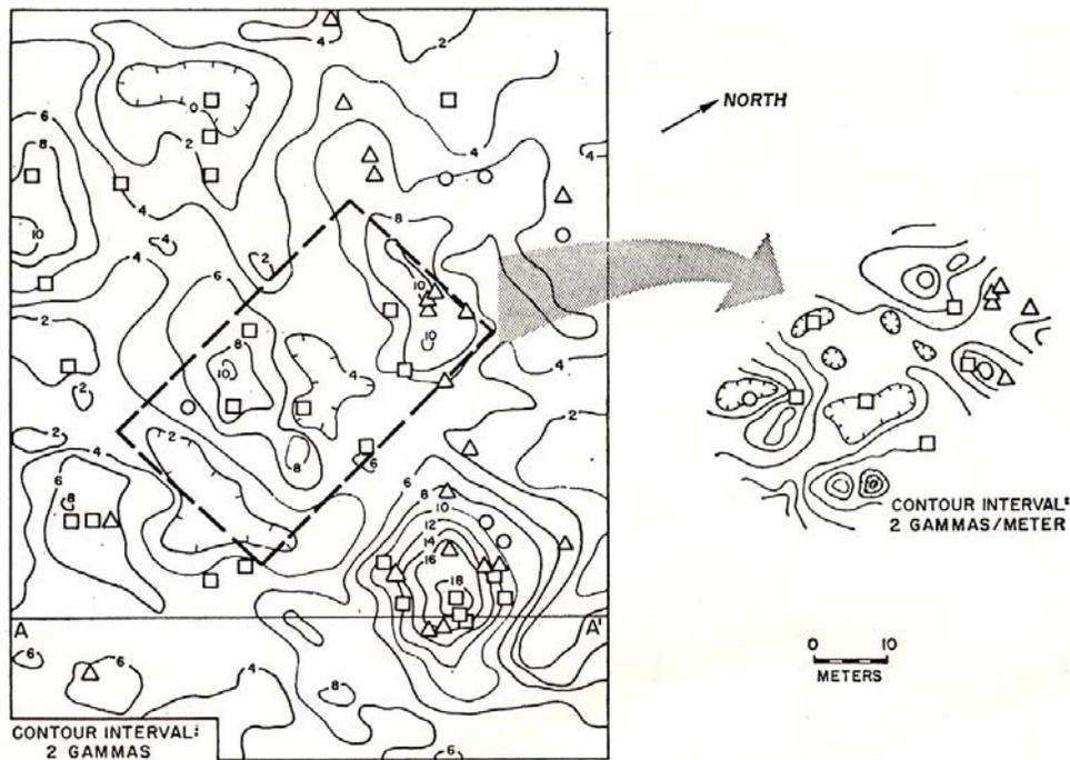
Fig. 8. Magnetic contour maps (grid 16: Zona Casa Bianca, plain of Sybaris, October 1964) over a complex of ruins, and results of drilling. (Left) Plot of total intensity. (Right) Plot of the difference between results of two surveys made at 0.5 meter and 1.5 meters above ground surface, respectively, in an area corresponding to the rectangle bounded by dashed lines in the plot at left. (Circle) No results; (squares) drill stopped by wall; (triangles) resistance from friable material.
