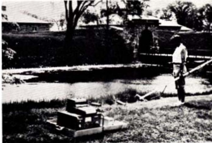
Fig. 2. A differential rubidium magnetometer in use at Fort Lennox, Quebec. The equipment at left makes recordings from the cylindrical sensors on the ground and on the hand-held staff.
