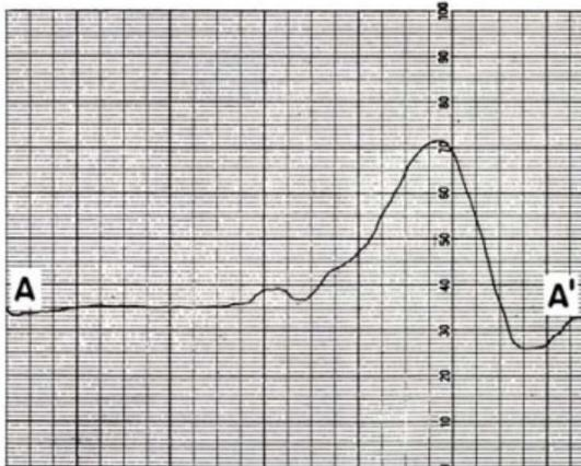
Fig. 7. Differential magnetometer profile recorded over a large anomaly of grid 16. Full scale represents 30 gammas.
