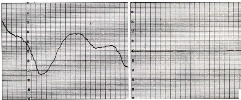
Fig. 3. Rubidium magnetometer recordings from the plain of Sybaris, made with both sensors in a fixed position. Full scale represents 1 gamma; duration of each recording shown, about 7.5 seconds. (Left) Single sensor recording of typical daytime micropulsations. (Right) Differential magnetometer recording made during the same activity, with almost complete cancellation of time variations.
